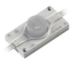
The MSL-1-450 is a maxi range LED module for sidelight in the OZ LED Lighting range. The MSL-1-450 best operates in the 150-300mm depth range for light boxes and commercial lighting. The MSL-1's special lens design with a beam angle of  $15^{\circ}$  x  $55^{\circ}$  allows for even side illumination within the light box.
