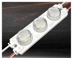
The MSL-3 is a solid LED module for side light in the OZ LED Lighting range. The MSL-3 best operates in the 50-120mm depth range for light boxes and commercial lighting. The MSL-3's special lens design with a beam angle of 10° x 65° allows for even illumination within the light box.
