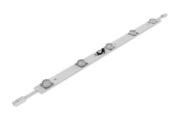
The MSL-5 is a solid LED module for side light in the OZ LED Lighting range. The MSL-5 best operates in the 100-400mm depth range for light boxes and commercial lighting. The MSL-5's special lens design with a beam angle of 15° x 45° allows for even illumination within the light box.
