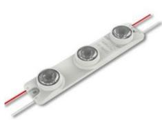
light in the OZ LED Lighting range. The MSL-3-650 best operates in the 120-300mm depth range for light boxes and commercial lighting. The MSL-3's special lens design with a beam angle of 15° x 45° allows for even illumination within the light box.
