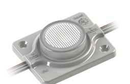
The MSL-1-150 is a mini range LED module for side light in the OZ LED Lighting range. The MSL-1-150 best operates in the 50-150mm depth range for light boxes and commercial lighting. The MSL-1's special lens design with a beam angle of  $15^{\circ}$  x  $25^{\circ}$  allows for even side illumination within the light box.
